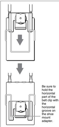
After attaching the belt clip, insert the shoe mount adapter between the portable diversity tuner (URX-P1) and the belt clip, with the vertical parts of the belt clip aligned with the two vertical parallel grooves on the shoe mount adapter. Then, push the shoe mount adapter in the direction of the arrow, and then catch the horizontal part of the belt clip with the horizontal groove on the shoe mount adapter to hold the belt clip in place.
